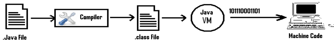
Fig 1.1 How Java Source code converts to Machine CODE
